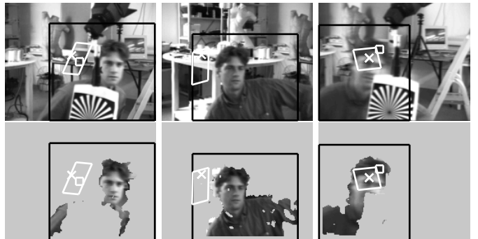
Figure 5: Resulting target pixels as extracted by the system (after integration and update) from the sequence shown in the top row. Using motion detection and an affine image velocity model for the target we can find areas that belong to the target such that occluding objects are removed and a correct pursuit is performed although we have partial occlusion. The pursued target is marked by the small rectangle. The small rectangle marks a fix point on the background as computed by the optokinetic mechanism. The pursuit is performed at 25 Hz, and shown are every 60 th frame.
